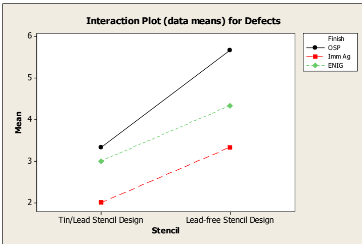
Figure 7. Interaction Plot for Defects.
